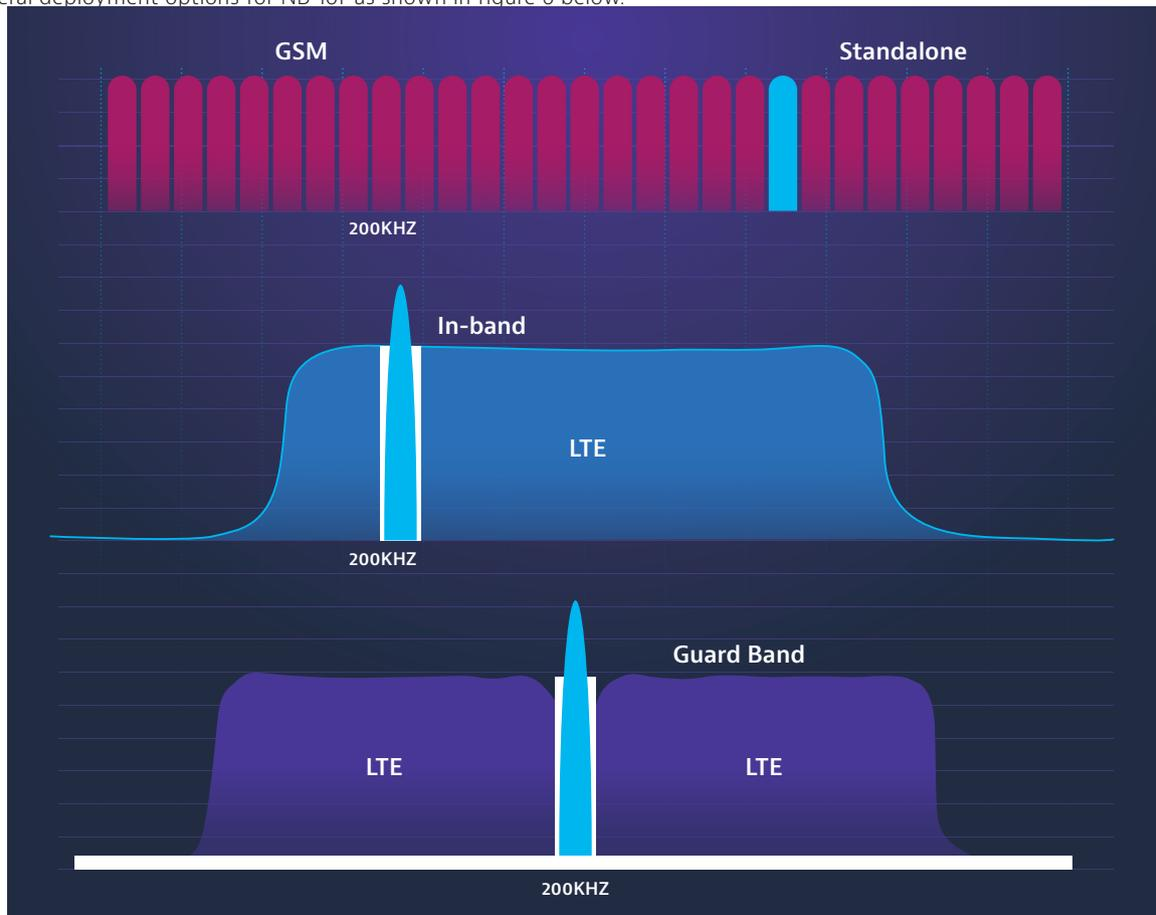
Figure 6: Deployment options for NB-IoT
