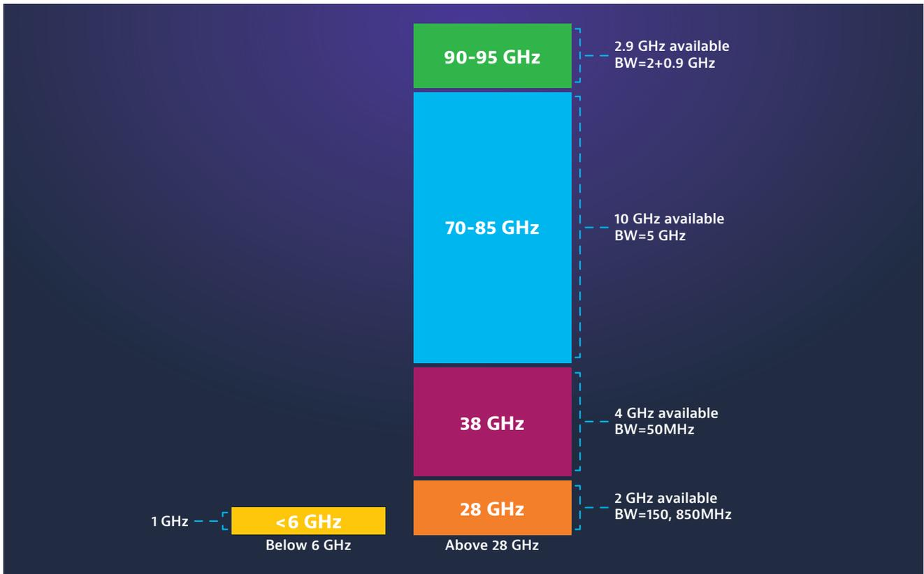
Fig 3: mmWave spectrum comparison with sub 6GHz
