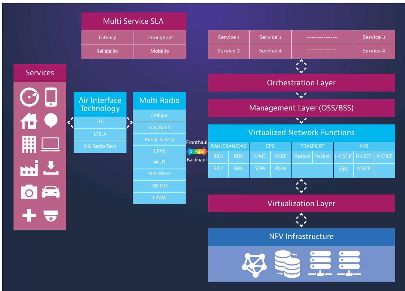
Figure 9: Virtualized Network with multiple network slices for multiple services
